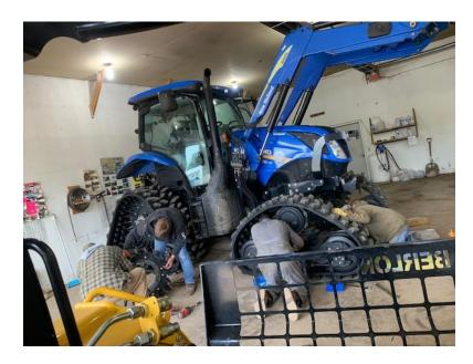
Pictured are Jim McDowall, Ron Fetkenuer, Doug Brunnner and Jim Becker switching from Soucy Tracks to tires for the summer grading season. Photo taken by Rick Fetkenheur behind the controls of the skid steer.
